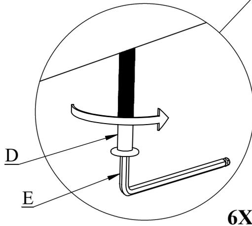
DO NOT TIGHTEN BOLT COMPLETELY
