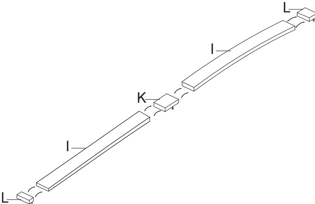
**Step 9.** Attach the Curved Slats pressing the Center Plastic Connectors and End Caps firmly into place.
