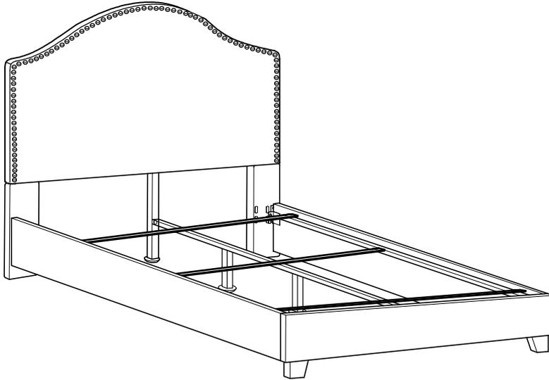
**Step 8.** Insert the ends of Curved Slats (Part I) into Center Plastic Connector (Part K) and End Caps (Part L). Repeat this step for all Curved Slats.
