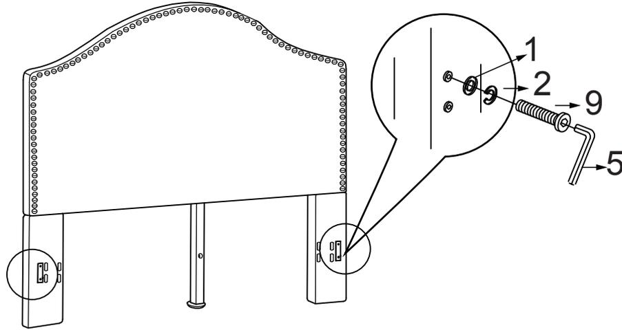
**Step 4.** Attach Side Rails (Part M) to the headboard and footboard as shown.
