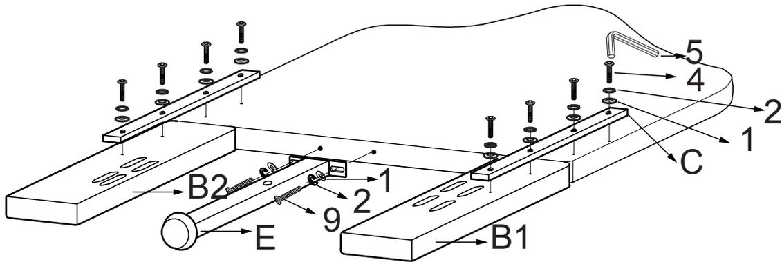
**Step 2.** Insert Wood Dowel (Part 10) into Wood Leg (Part G). Add Spring Washer (Part 2), and Flat Washer (Part 1) to Bolt (Part 8). Use Allen Key to attach the legs to the footboard.
